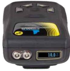
The twin shot injection moulded enclosure has a soft but durable TPE outer skin which is comfortable to hold and protects against bumps while the hard internal shell offers maximum strength and environmental protection certified to the demanding US MIL STD 810G standard.
