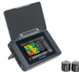
The Pundit Pulse Echo transducer is a shear wave transducer designed for single-handed and two-handed operation. It is particularly suited to testing where access is limited to a single side. It can be used
