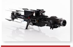
Operating height 2600 m Operating temperature --30 °C - +50 °C Operating speed 15 m/s
